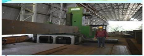
★ End Milling machines are used in Milling Application such as Profile Milling, Tracer Milling, Face Milling etc.
