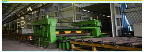
The Plate straightening machine is used to straightening the 6mm to 40mm size plates which is used to Fabrication of Girders. This machine is located at Girder Shop. The average cost of the machine is 4 Crore.
