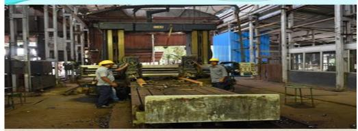
There are total 2 Nos. of Planning machine are available in this Workshop. Cooper Double Column Planning machine is use for machining work of 52kg and 60 Kg tongue rails and stocks rails for Fabrication of 1 in 8.5 curve switch and HEC Double Column Planning machine is use for machining of 52kg and 60 Kg tongue rails and stocks rails for Fabrication of 1 in 12 curve switch.
