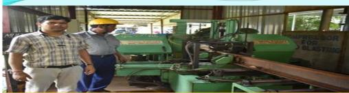
The said machine is very useful for cutting of Rails for production of glued Joints and others allied components like SSD Fitting materials, Bunch cutting of various types of round bars, angles etc.
