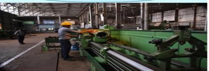
A Lathe is a machine tool that rotates a workpiece about an axis of rotation to perform various operations such as cutting, drilling, facing, knurfling, grooving, turning, threading & taper turning etc. with tools that are applied to the workpiece to create an object with symmetry about the axis.
