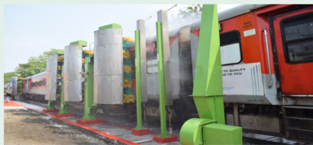
Automatic Coach Washing Plant at Padmapukur, Shalimar
