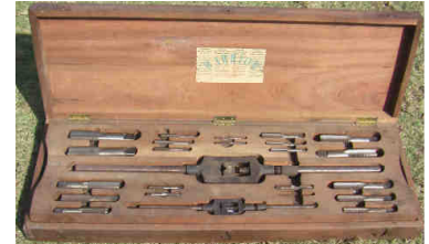
TAPS & DIES (Made in England) to cut thread over and inner side of the water Pipes Received on - 24.02.2007
