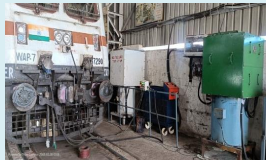
HLC full load test set-up
